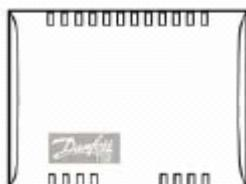
The programmable room thermostat controls the boiler, telling it when you require central heating and hot water. It has the facility to give several on/off times. Temperatures can also be selected for each on/off time. When the heating is selected on it will operate until the set temperature is achieved. Note that the temperature is measured by the remote temperature sensor located typically in the living room or hall. The remote temperature sensor should not be
